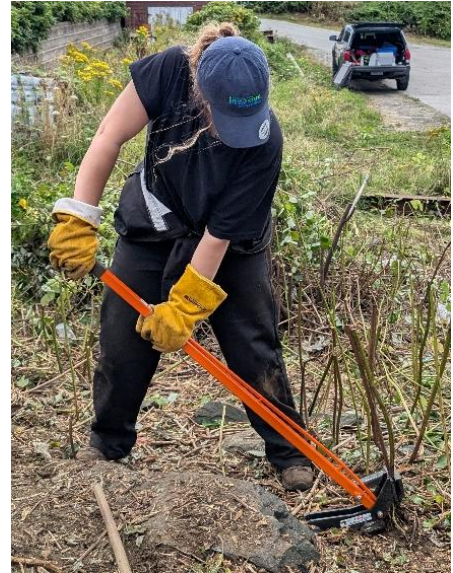
Photo 3. An Extractigator being used to remove an invasive shrub.
